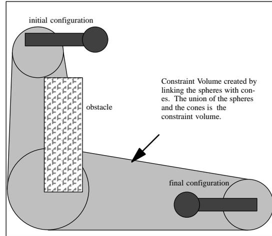
Figure 4. Constraint Volume specified by placing a set of circles (spheres for 3d) of various sizes.
